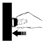
The control must be pushed in to set only from the OFF position. When the control is in any position other than OFF, it may be turned without pushing it in.
